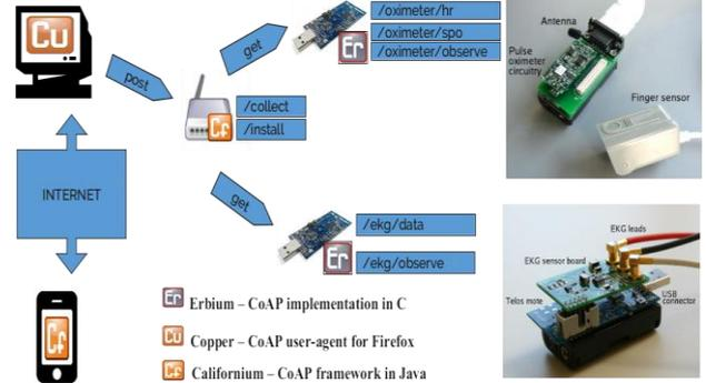
Figure 2 Architecture of the CoAP-based Wireless Sensor Network used as testbed
