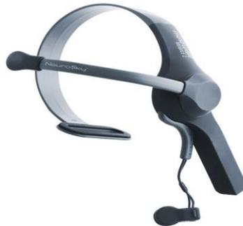
**Fig. 3.** The NeuroSky MindWave Mobile 2 used in the system.
