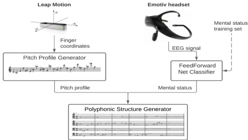
**Fig. 2.** System architecture
